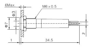
6 MAX: means the panel thickness, the max thickness for the panel no more than 6mm.
