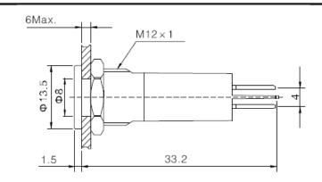
6 MAX: means the panel thickness, the max thickness for the panel no more than 6mm.
