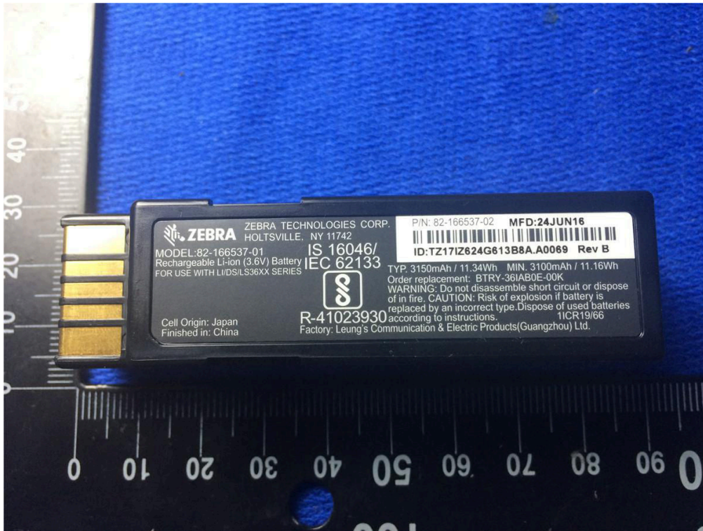
Battery (82-166537-01 3,6V 3150mAh/11,34Wh(TYP) 3100mAh/11,16Wh(Min))
