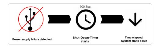
If the StromPi 3 now detects a power failure, the timer starts. After 10 minutes the StromPi 3 will then disconnect the power supply to the Raspberry Pi. Additionally we provide a script that can detect a power failure either via the serial console or via a GPIO pin and then shut down the Raspberry Pi safely. The shutdown timer can be set in the config script by **Shutdown Timer**.
