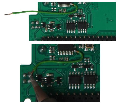
Finally the other end of the cable is soldered to the lower solder pad.
