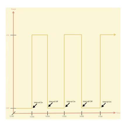
The interval function allows you to define time intervals in which the Raspberry Pi is switched off and on again with the help of the StromPi 3.You can activate and configure this function in the config script by **Timer**.
