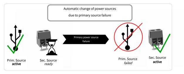
In total there are six different modes possible. The primary power source is the main power source. The secondary power source will take over when the primary source fails.
