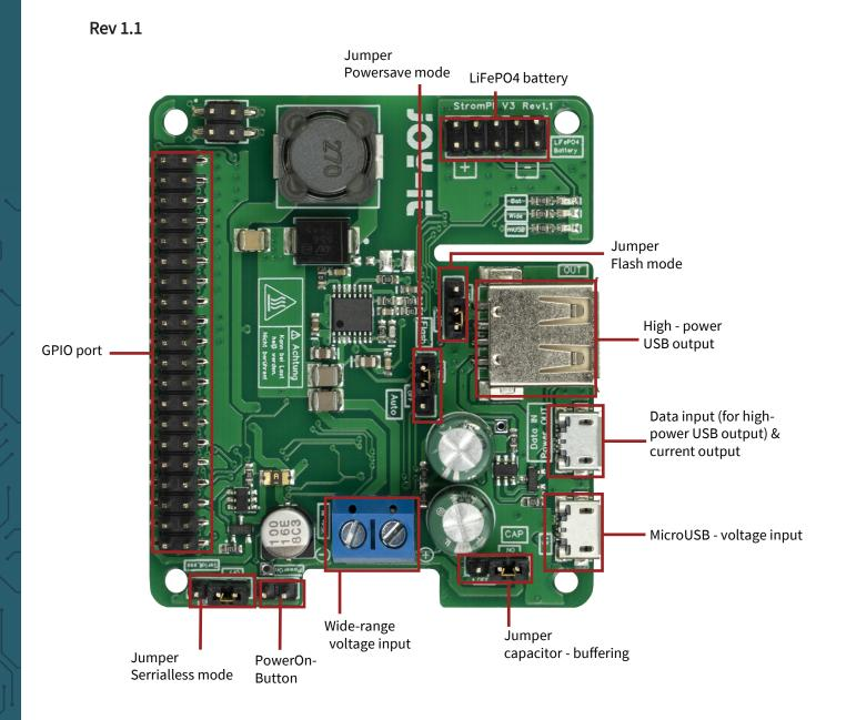
The newly added serialless jumper connects the GPIO 21 (pin 40) of the Raspberry Pi to a GPIO of the microcontroller when set to "ON". The serialless function must still be activated as usual in the configuration of the StromPi 3.
