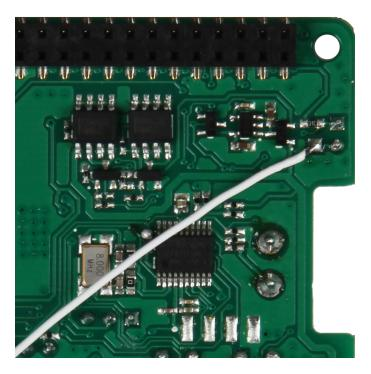
Solder the other end of the cable as shown in the picture below one of the GPIO pins.
