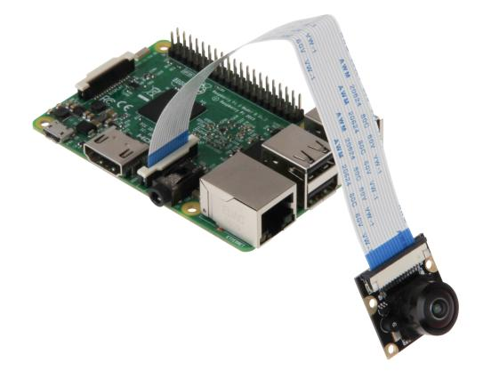
Connect the camera module, as seen in the image, with the shipped ribbon cable to the CSI interface of your Raspberry Pi.
