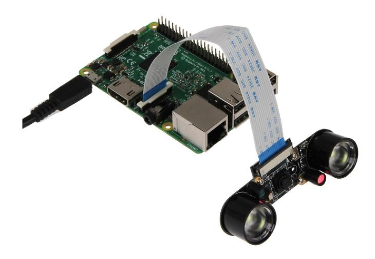
Connect the camera module, as seen in the image, with the shipped ribbon cable to the CSI interface of your Raspberry Pi.
