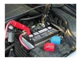
CONNECT THE EMERGENCY / BOOSTER CABLE TO THE BATTERY TERMINAL.
