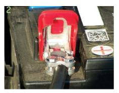
2. INSERT THE STRIPPED CABLE INTO THE RIGHT PLACE AND TIGHTEN THE SCREW TO THE PLATE WITH A SCREWSPANNER #10
