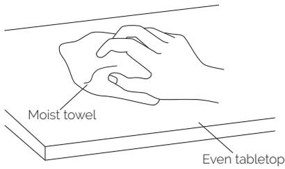
First, use a moist towel to wipe the surface of the table, then place the sheet material for the wings and tail separately onto the tabletop with the unprinted side facing up.
