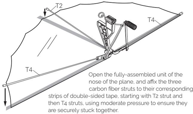
Open the fully-assembled unit of the nose of the plane, and affix the three carbon fiber struts to their corresponding strips of double-sided tape, starting with T2 strut and then T4 struts, using moderate pressure to ensure they are securely stuck together.
