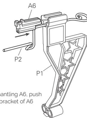
\*When dismantling A6, push the bottom bracket of A6 outward.
