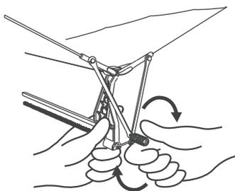
Hold A5 and turn the crank clockwise about 50 times.
