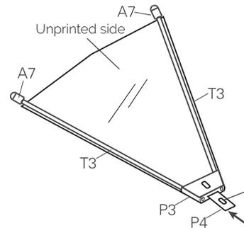
Insert T3 carbon fiber struts into their corresponding holes in P3 and attach A7 to the outer ends. Insert copper chip P4 into the slot at the other end of P3, then attach the assembled unit to the tail sheet.
