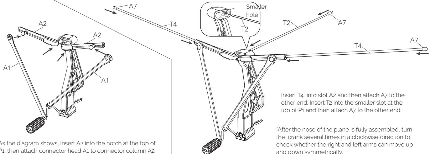
As the diagram shows, insert A2 into the notch at the top of P1, then attach connector head A1 to connector column A2.
