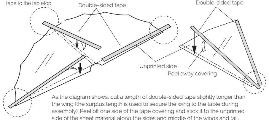
As the diagram shows, cut a length of double-sided tape slightly longer than the wing (the surplus length is used to secure the wing to the table during assembly). Peel off one side of the tape covering and stick it to the unprinted side of the sheet material along the sides and middle of the wings and tail.
