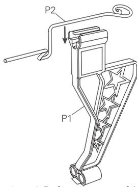
Insert crank P2 from the nose of the plane into the bottom of slot P1 as shown in the diagram, with the bend kept vertical and pointing downward.
