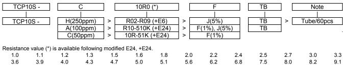
Note\*: When ordering, additional ohm resistance notation is recommended for keeping out of misunderstanding.
