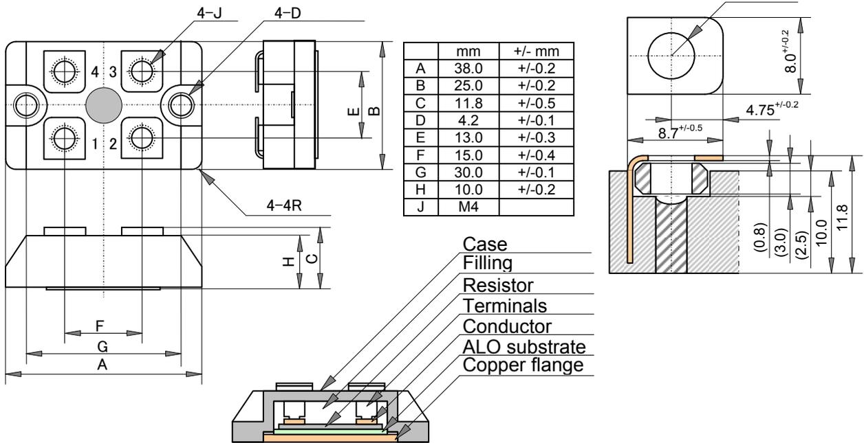
Note: The depth of the screw hole is about 4.3mm from the surface of the terminal plate.
