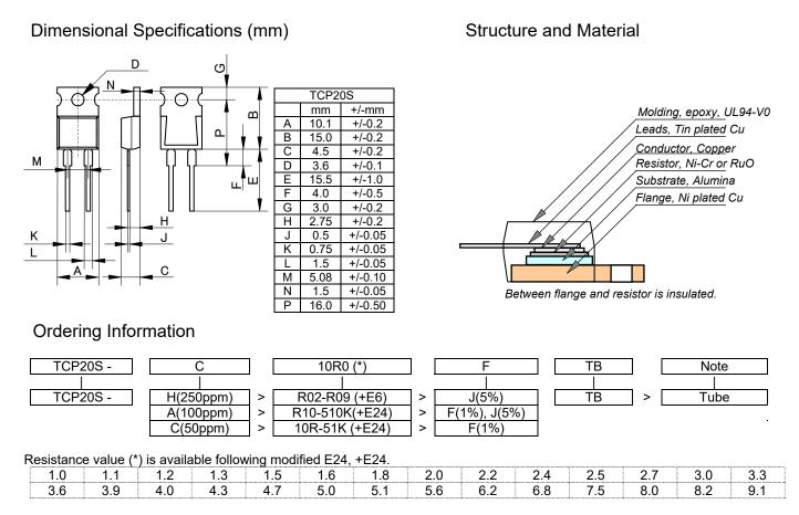
Note\*: When ordering, additional ohm resistance notation is recommended for keeping out of misunderstanding.
