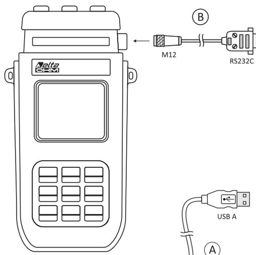
**A** USB connection to PC using type A USB - M12 cable, code HD2110USB. **USB drivers are required.**
