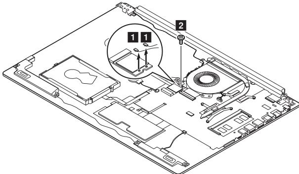
In step ■, unplug the jacks by using the removal tool antenna RF connector (P/N: 08K7159), or pick up the connectors with your fingers and gently unplug them in the direction shown by the arrows.
