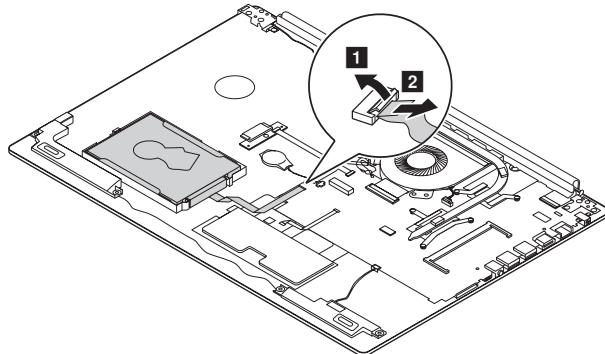
**When installing:** Make sure that the HDD board connector is attached firmly.
