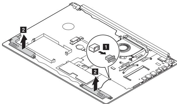
**When installing:** Make sure that the connector is attached firmly.
