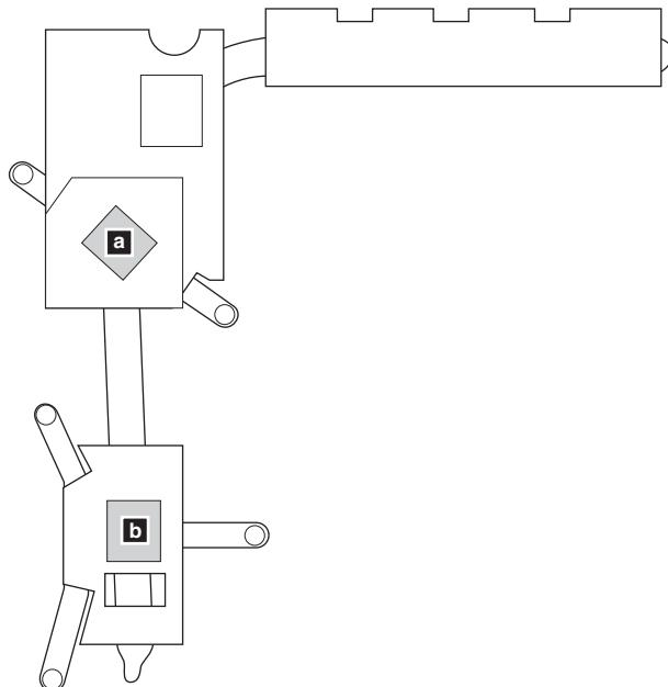
**When installing:** Before you attach the fan assembly to the computer, apply thermal grease, at an amount of 0.2 grams, to the **a b** part shown in the figure above. Either too much or too little grease application can cause a thermal problem due to imperfect contact with a component.
