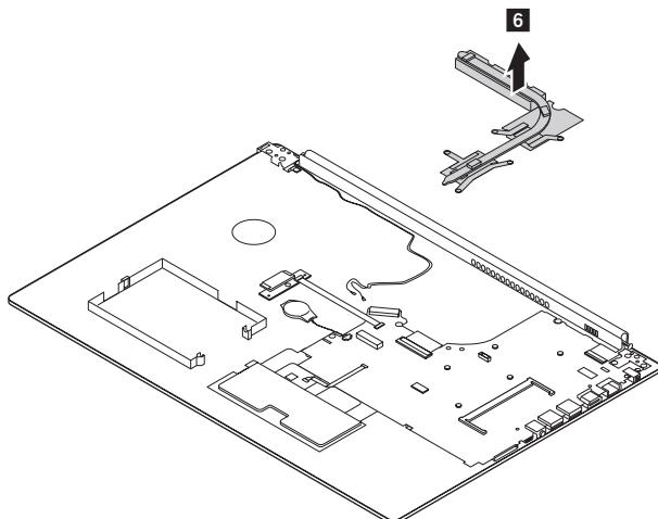
Figure 8. Removal steps of fan assembly and Heat Sink assembly (continued)
