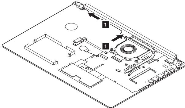
**When installing:** Route the antenna cables along the cable guides. As you route the cables, make sure that they are not subjected to any tension. Tension could cause the cables to be damaged by the cable guides, or a wire to be broken.
