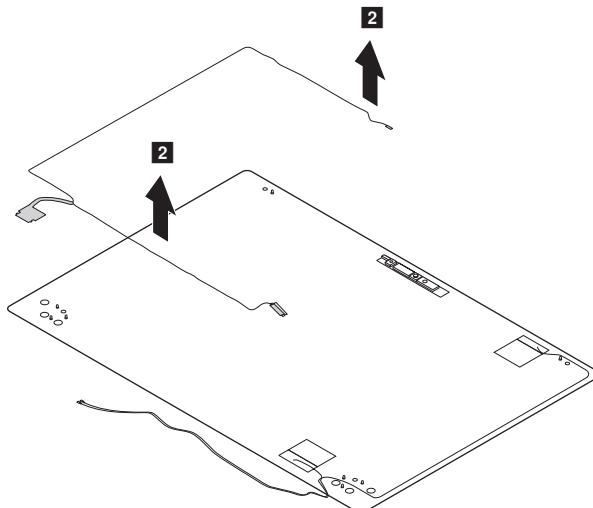
**When installing:** Make sure that the connector is attached firmly and that you do not pinch the antenna cables when you attach the LCD assembly. Route the LCD cable along the cable guides.
