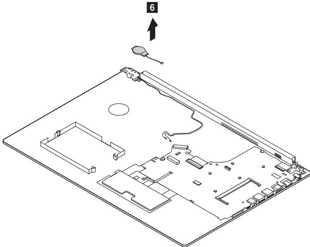
**When installing:** Make sure that the connector is attached firmly.
