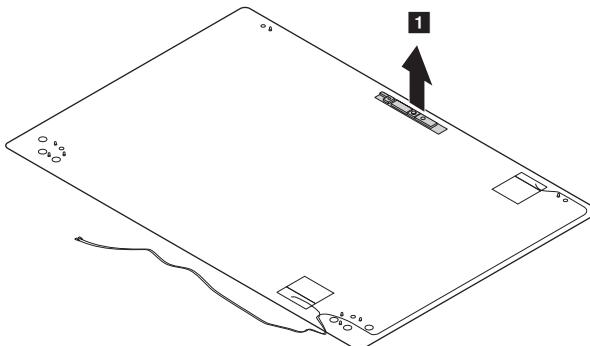
**When installing:** Stick the integrated camera to the top center of the LCD cover and adjust its placement to make sure the connector is attached firmly.
