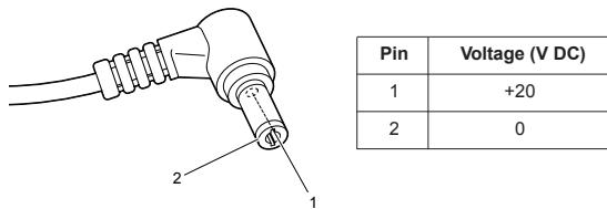
**Note:** Output voltage for the AC adapter pin No. 2 may differ from the one you are servicing.
