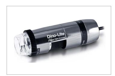
With the use of the latest, cutting-edge optics, a brand new 5 megapixel sensor and several special features such as flexible LED control (FLC), Automatic Magnification Reading (AMR) and full aluminum body, the Dino-Lite AM7515MZT is a marvel of technology and the best choice for the highdemanding professional.
