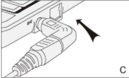
1. When you want to charge or supply power to laptop, connect the AC plug into the wall socket (picture A). Choose the right tip for your laptop, such as N04, join it with the DC output (picture B), connect the joint DC tip to the laptop then it can be used. (picture C)
