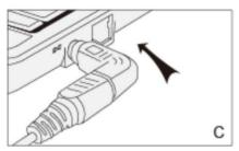
When you want to charge or supply power to laptop, connect the AC plug into the wall socket (picture A). Choose the right tip for your laptop, such as NO4, join it with the DC output(picture B), connect the joint DC tip to the laptop then it can be used. (picture C)
