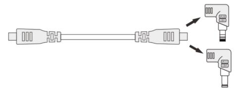
Caution: This adapter supports voltage output ranging from 14.5-24 volts. Please be informed that using this adapter to charge a notebook outside of the 14.5-24 volts range may damage the notebook.
