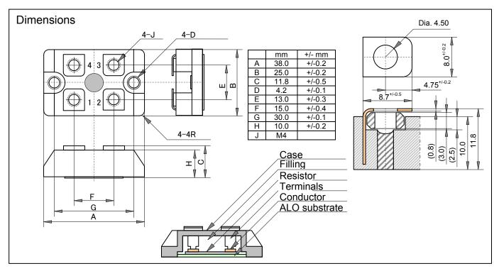
Note: The depth of the screw hole is about 4.3mm from the surface of the terminal plate.
