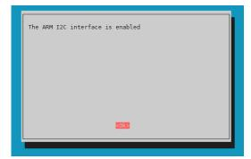
You have now successfully activated I2C. The analog-to-digital converter is now accessible under the I2C address 0x48, which is set by default for this sensor. The I2C address will be different if you have already configured it before configuring your Raspberry Pi.
