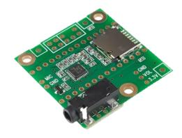
This audio board is an addon for the development cards Teensy 3.0 and 3.1. The audio board is a user-friendly solution to provide your teensy project with high quality audio (16 bit, 44.1 kHz).
