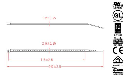
Material: Nylon 66 UL 94V-2 Tolerance: As Figure
