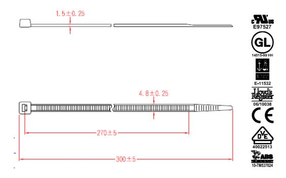
Material: Nylon 66 UL 94V-2 Tolerance: As Figure
