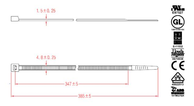
Material: Nylon 66 UL 94V-2 Color: Black Tolerance: As Figure
