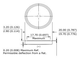
0.10 (0.004) Minimum Ref. (Applies to top edge of gasket or edge of crimp, whichever is higher.)
