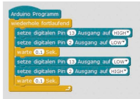
The `02mb1ock` program lets two LEDs to flash alternately.
