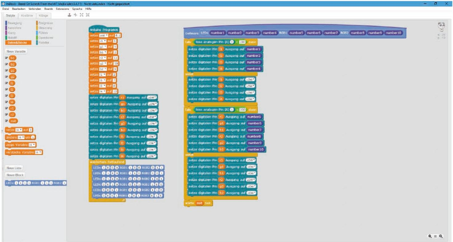
The program 21mblock flashes with a self-defined block of LEDs.
