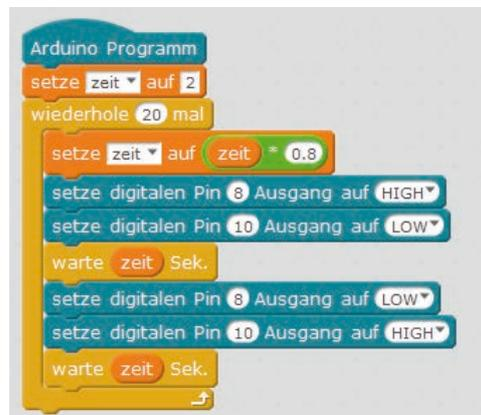
The program `04mblock` makes two LEDs flash.**How the program works**
