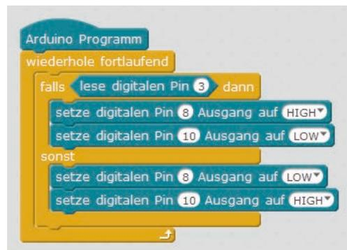
The 05mb1ock program switches the LEDs when the button is pressed.
