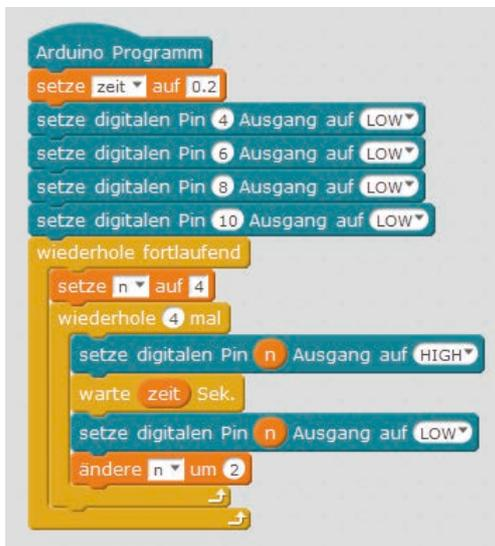
The program `09mb1ock` controls a chaser light consisting of four LEDs on the angel wing.
