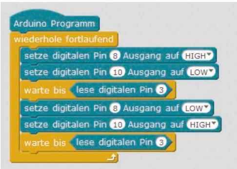
The 06mb1ock program switches two LEDs with one button.
