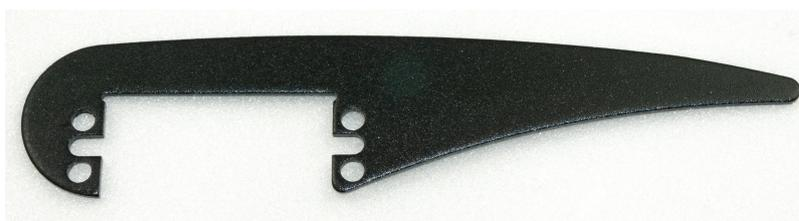
Figure 85: 3x leg "Tibia" left + 3x leg "Tibia" right (always take care to round off the edges)
