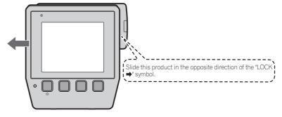
2 Remove this product so that the hooks on the Installation Bracket disengage from the slots on this product.
