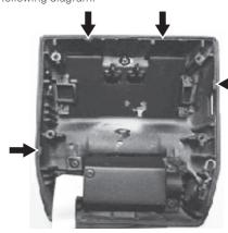
The hooks can be released with a flathead screwdriver.
