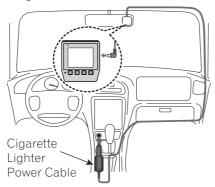
↑ The power terminal will be extremely hot immediately after using the cigarette lighter. The tip of the Cigarette Lighter Power Cable may melt or short circuit if it is plugged in while hot. Wait for the terminal to cool before plugging in the Cigarette Lighter Power
