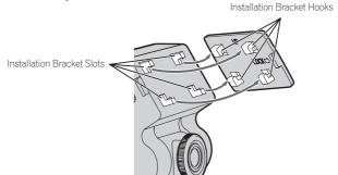
Reverse the steps to reattach this product. Line up and fit together the hooks on the Installation Bracket with the slots on this product, then slide this product to the right as viewed from the LCD (the direction indicated by the "LOCK\*) symbol on the Installation Bracket).
