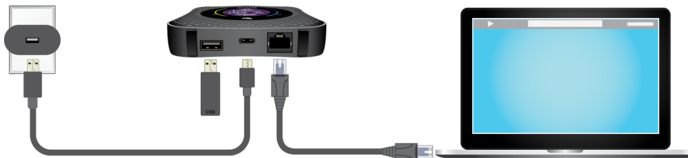
Figure 6. Ethernet offloading with AC charging and a USB storage device
