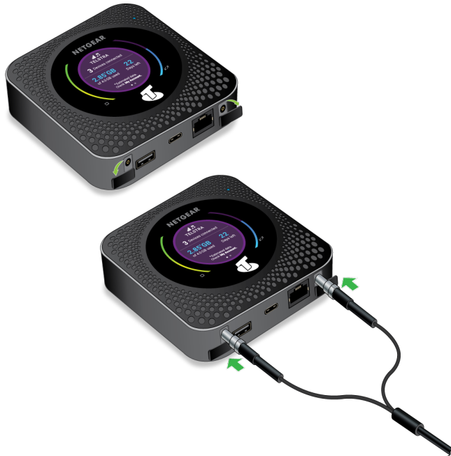
Figure 4. External antennas with TS9 connectors
