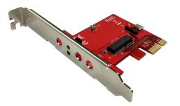
Utilize Advanced PCIe base and USB base M.2 E Key and A-E Key WiFi Wireless Module on Industrial Computer PCIe x1 Slot!
