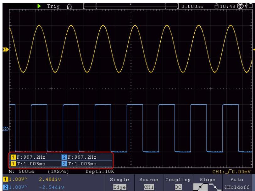
Figure 4-14 Automatic measurement
