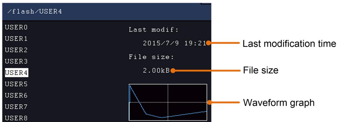
If a USB device is connected, and you want to save the waveform to it, select **Memory** in the right menu as **USB**. The instrument lists a directory of the folders and files on the USB memory device. Select a folder or file using the **M** knob to scroll up and down the list. To enter the current folder, select **Change Dir** in the right menu, select it again to return to the upper directory.
