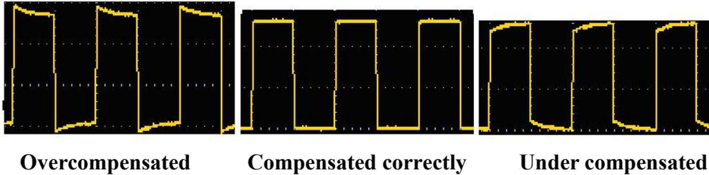
Figure 3-7 Displayed Waveforms of the Probe Compensation
