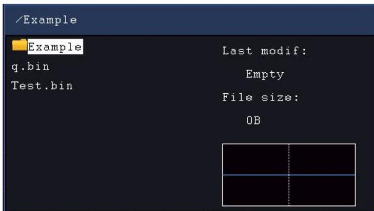
Enter the desired storage path, select **Save** in the right menu, an input keyboard pops up, input the file name, choose **↵** in the keyboard to confirm. The waveform is saved as BIN file in the folder.
