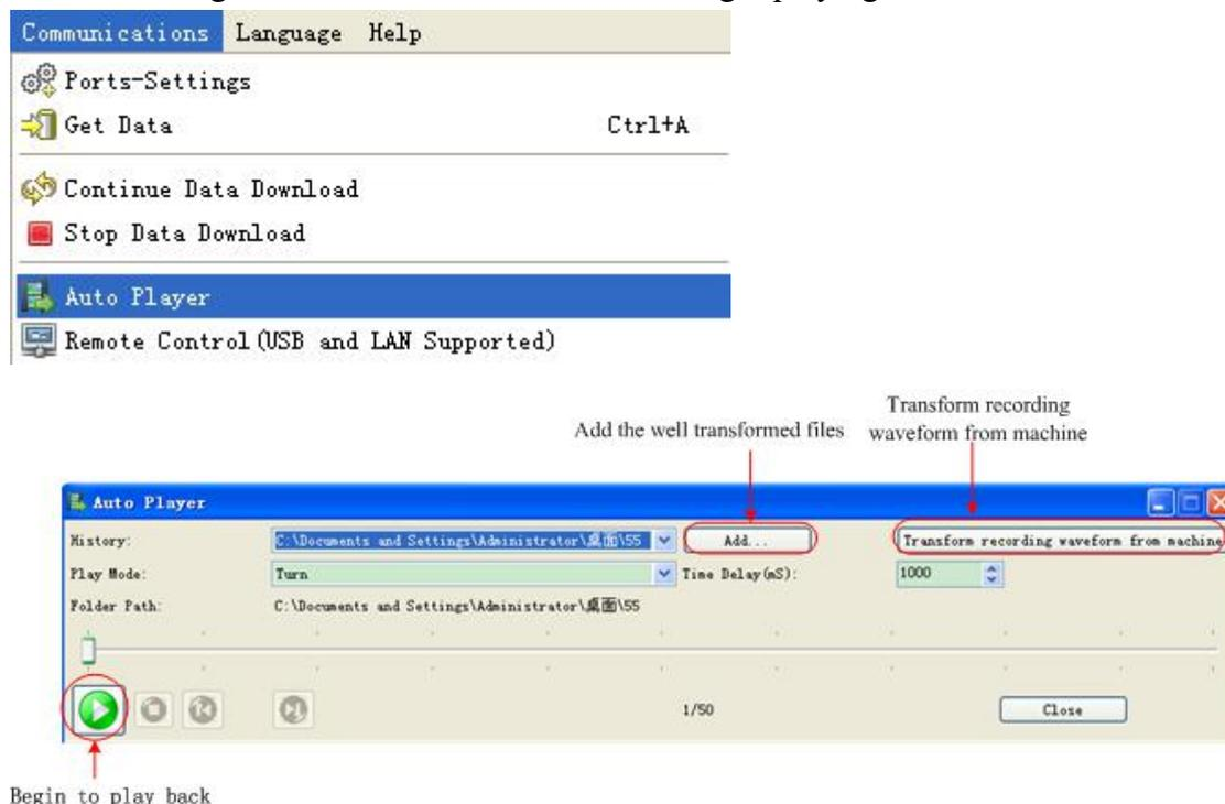
Figure 4- 13: Play back waveform by software
