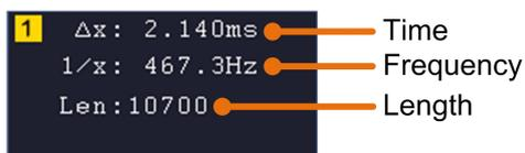
**Note:** If "Out Of Limits" appears in the information or a message "Waveform points beyond the limit." appears on the screen, that means the length of the cloned waveform exceeds the limit. When the source is CH1 or CH2, the maximum length is 2M; When the source is CH1&CH2, the maximum length is 1M. Push the **Acquire** button, select **Length** in the bottom menu, and set the record length to a smaller value.
