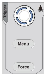
Figure 3- 13 Trigger Control Zone
