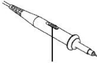
Figure 3-9 Attenuation Switch
