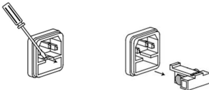
3. Replace the fuse with a new one, which should match with the rating; install it into the fuse box and then push the fuse box back on to the rear panel.
