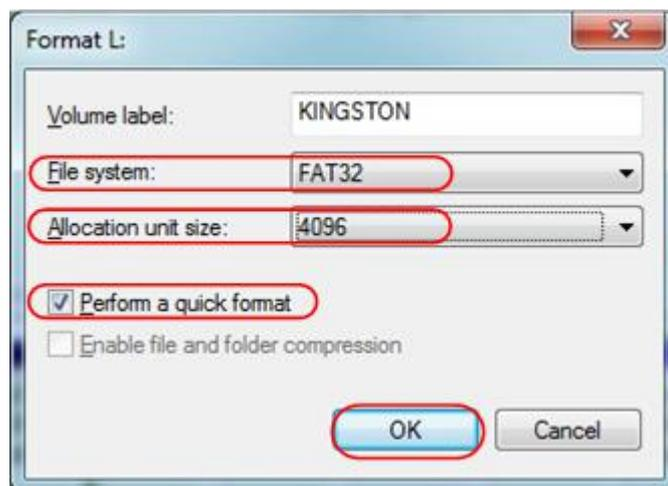
Figure 4- 5: Formatting the USB disk setting
