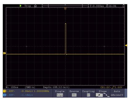
Figure 8-3 Capturing a Single Signal
