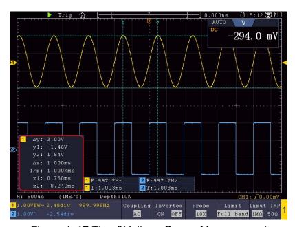
Figure 4-17 Time&Voltage Cursor Measurement
