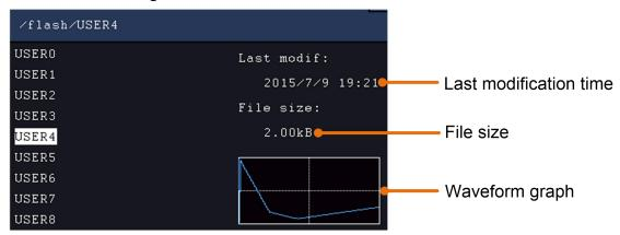
If a USB device is connected, and you want to save the waveform to it, select **Memory** in the right menu as **USB**. The instrument lists a directory of the folders and files on the USB memory device. Select a folder or file using the **M** knob to scroll up and down the list. To enter the current folder, select **Change Dir** in the right menu, select it again to return to the upper directory.
