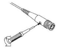
Figure 3-8 Adjust Probe
