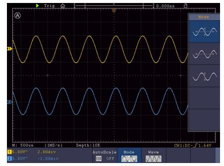
Figure 4-18 Autoscale Horizontal-Vertical multi-period waveforms
