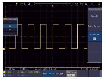
Figure 8-5 Reduce Noise level by using Average function
