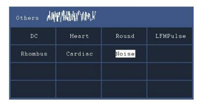
(4) Turn the M knob to select the desired waveform (or touch). E.g. select Noise. Select Select to output the noise waveform.
