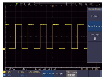
Figure 8-4 Signal with Noises
