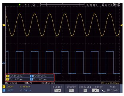
Figure 4-14 Automatic measurement
