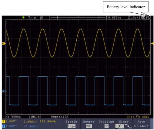
Figure 11-1 Battery level indicator
