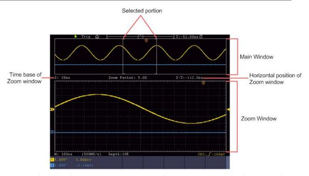
In normal mode, the **Horizontal Position** and **Horizontal Scale** knobs are used to adjust the horizontal position and time base of the Main window.
