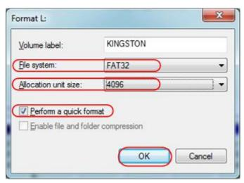
Figure 4-5: Formatting the USB disk setting
