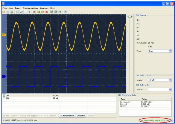
Figure 7-1 Connect with PC through USB port
