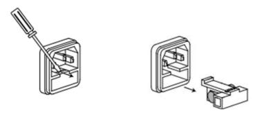
3. Replace the fuse with a new one, which should match with the rating; install it into the fuse box and then push the fuse box back on to the rear panel.
