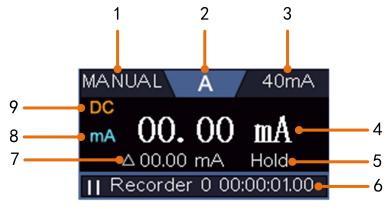
Figure 6-2 Multimeter Information Window
