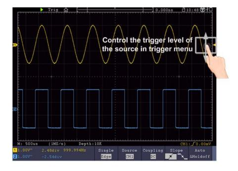
• Set the horizontal position (Horizontal Position knob): Swipe left or right on the display area.
