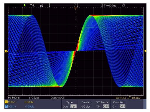
Figure 4-2 The color temperature function is on
