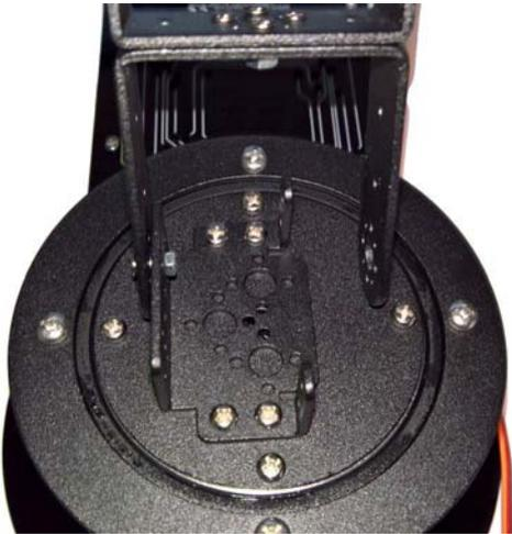
And place the servo and fix it with 4 screws and nuts.
