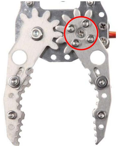
Mount a servo-lever to the angle and fix it to the servo with a screw.
