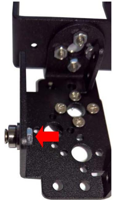
Place the servo motor and mount it with 4 screws and nuts. Mount it to the robot arm with screws on both sides.
