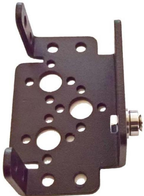
Mount a bearing to the first angle-plate.
