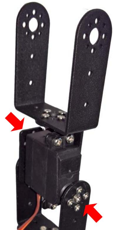
Place two servo holders on each other and fix it with screws and nuts.
