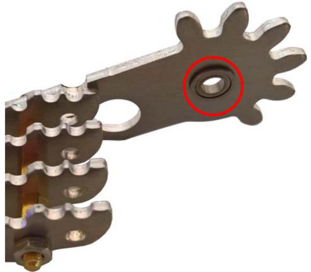
Mount the first claw on the servo with a washer and a nut.
