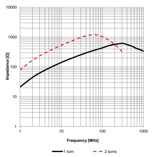
CHECKED GENERAL TOLERANCE PROJECTION METHOD CREATED Würth Elektronik eiSos GmbH & Co. KG **EMC & Inductive Solutions** KaS DIN ISO 2768-1m Max-Eyth-Str. 1 74638 Waldenburg STAR-TEC Snap Ferrite with safety Tel. +49 (0) 79 42 945 - 0 key technology ORDER CODE 74271211 www.we-online.com eiSos@we-online.com DATE (YYYY-MM-DD) BUSINESS UNIT STATUS PAGE 001.001 Valid 2/4 2018-02-20 eiSos **WÜRTH ELEKTRONİK**
