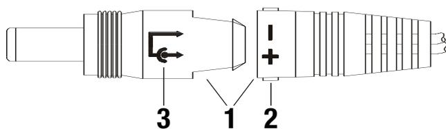
1. To connect for desired polarity, both plug ends are clearly marked.
