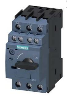
Special type Circuit breaker size S00 for motor protection, CLASS 10 A-release 5.5...8 A N-release 104 A screw terminal Standard switching capacity with transverse auxiliary switches 1 NO+1 NC Ambient temperature -50 °C 500 switching cycles
