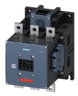
Power contactor, AC-3 225 A, 110 kW / 400 V AC (50-60 Hz) / DC operation 23-26 V UC Auxiliary contacts 2 NO + 2 NC 3-pole, Size S10 Busbar connections Drive: conventional screw terminal Auxiliary switch block 2 NO + 2 NC lateral, left + right Captive auxiliary switch, DIN 50012
