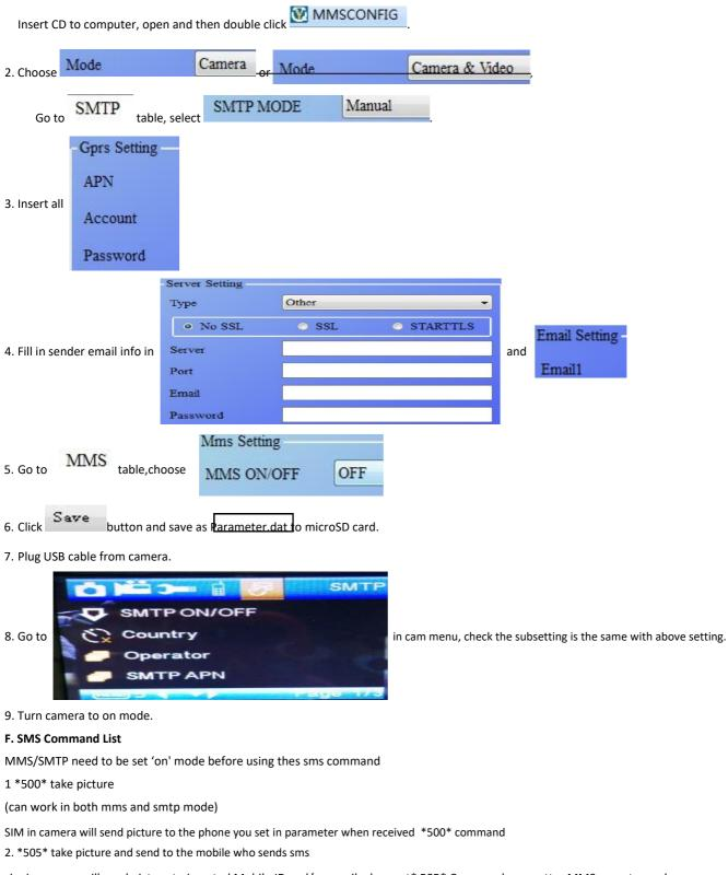
sim in camera will send picture to inserted Mobile ID and/or email when got\* 505\* Command, no matter MMS or smtp mode.
