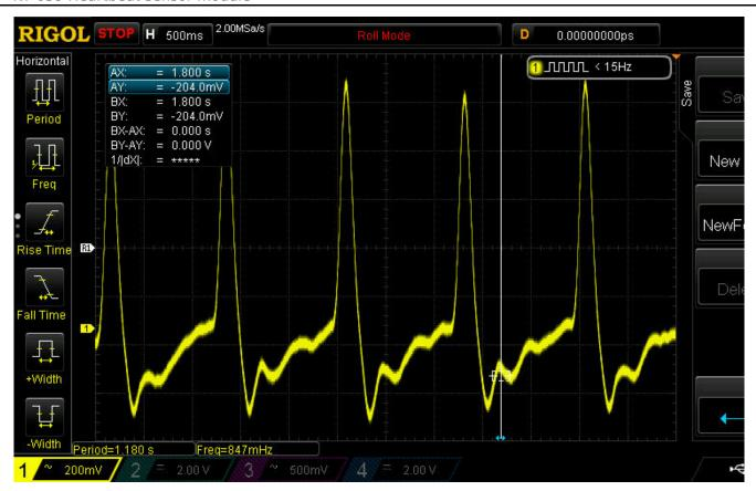
This shows, the changes of the voltage at the phototransistor - and with it the brightness change which comes from the flowing blood. The peaks above show the heartbeat. If you calculate the measured beats per recorded time, you will nearly get 71 beats per minute (bpm).
