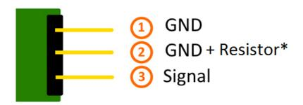
You can directly solder a resistor to the circuit board. In that case, the central pin (2), which includes the resistor, can be used.
