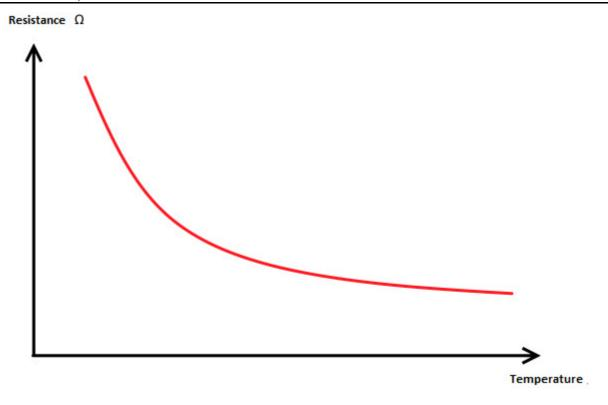
You can draw near to the resistant change via maths and convert it into a linear course. With that you can determine the temperature coefficient (addicted from resistant change to temperature change). With that you can determine the actual temperature if you know the current resistance.
