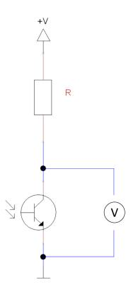
If you switch a resistor and a transistor in row, you will see a special behavior if you measure the voltage at the transistor: if much light shines at the transistor, you will measure a very low voltage (near 0V).
