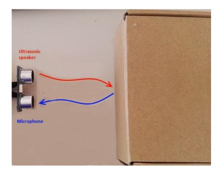
The Ultrasonicspeaker sends 8x 40KHz signals, which will be reflected by objects and recorded with the microphone, in this sensor module. Ultrasonic is being used because you are not able to hear it with the human sense of hearing (Human sense of hearing is nearly 20HZ - 22.000Hz).
