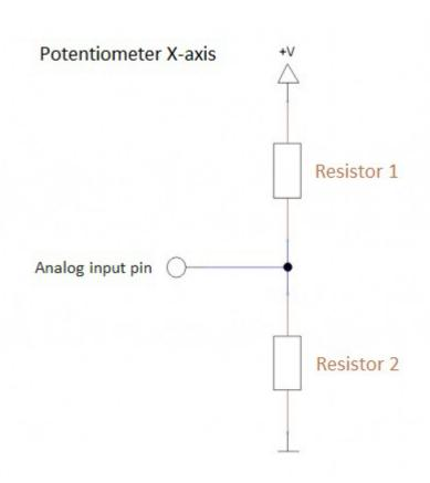
In the non-operating mode, the potentiometer is in the middle so that resistor1=resistor2, so that the voltage will equally split to both resistors - e.g. Measurement of +V=5V -> 2,5V.
