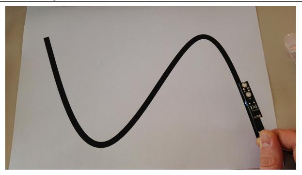
Condition 2: Line Tracker not on a line (reflecting area) [LED on the module: ON] [Sensor signal = Digital Off]
