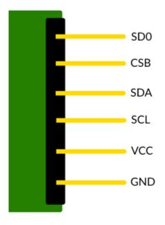
\*You can connect this sensor to 5V systems and to 3,3V systems. Please pay attention that only one of the power supply pins is connected to the desired voltage - you can get additional informations at the example below: Connection Arduino (5V) and Connection Raspberry-Pi (3,3V).
