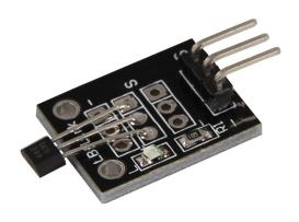
With this small Hall magnetic field sensor, you can detect magnetic fields using the sensor's digital output and the integrated status LED. When the sensor is held in a magnetic field, the LED lights up and the sensor output switches to low state.
