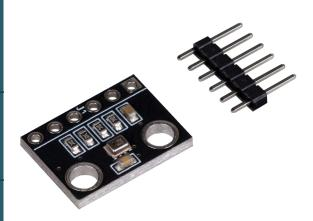
With this sensor board you can measure both air pressure and temperature. The sensor can be controlled either via I2C or via SPI.
