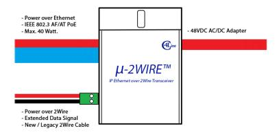
The µ-2WIRE™, model C4L6400M-2W-P is the Mini Size IP Ethernet over 2Wire transceiver. It support up to 200 Mbps data transfer speed for IP Intercom, IP Camera, IP Access Control, VoiP, Wi-Fi Network, Home Automation, Building Network application.
