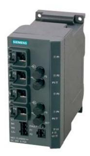
SIPLUS NET SCALANCE X204-2 -40...+60°C for medial exposure based on 6GK5204-2BB10-2AA3 . Managed IE switch, 4x 10/100 Mbit/s RJ45 ports, 2x 100 Mbit/s multimode BFOC, LED diagnostics, error signaling contact with set button, Redundant power supply, PROFINET IO device, network management, integr. redundancy manager, incl. electron. Manual on CD-ROM, C-plug optional
