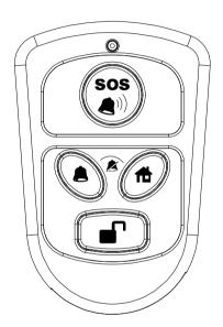
The button on the remote control can be configured as an Emergency Call or Panic button via the base unit.
