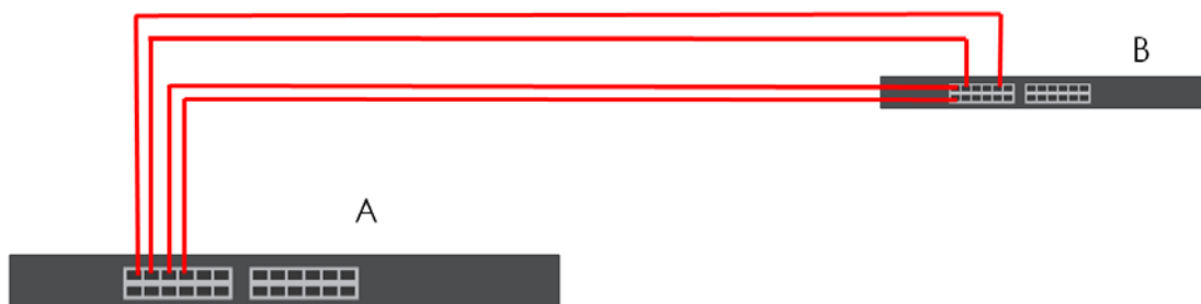
Figure 126 Trunking Example - Physical Connections
