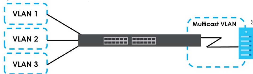
Figure 171 MVR Network Example
