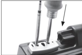
Place the handpiece on top of the new cartridge and press down slightly.
