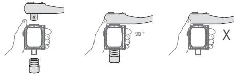
Use only suitable extensions, squares and ratchets. Connect all individual components centred, straight and precisely flush, otherwise there is a risk of damage.
