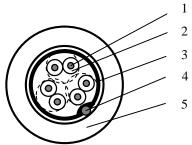
1. Conductor AWG24 (7xAWG32) tinned Cu
