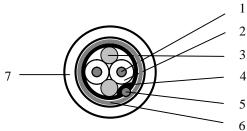
1. Conductor AWG20 (7xAWG28) tinned Cu
