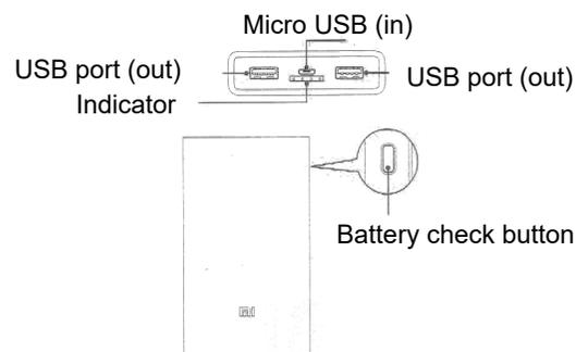
Note: the «battery check» button are not intended to turn on / off the device. This battery has the function of automatic detection of charging and discharging, so there is no need to constantly press the charge check button. In two minutes before the discharge, the amount of power LEDs are switched off.
