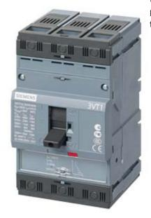
circuit breaker 3VT1 standard breaking capacity lcu=25kA, 415V AC 3-pole, line protection trip unit TM, LI In=20A rated current IR=16...20A overload protection II=200...300A, short-circuit protection without auxiliary release without auxiliary/alarm switch with front terminals
